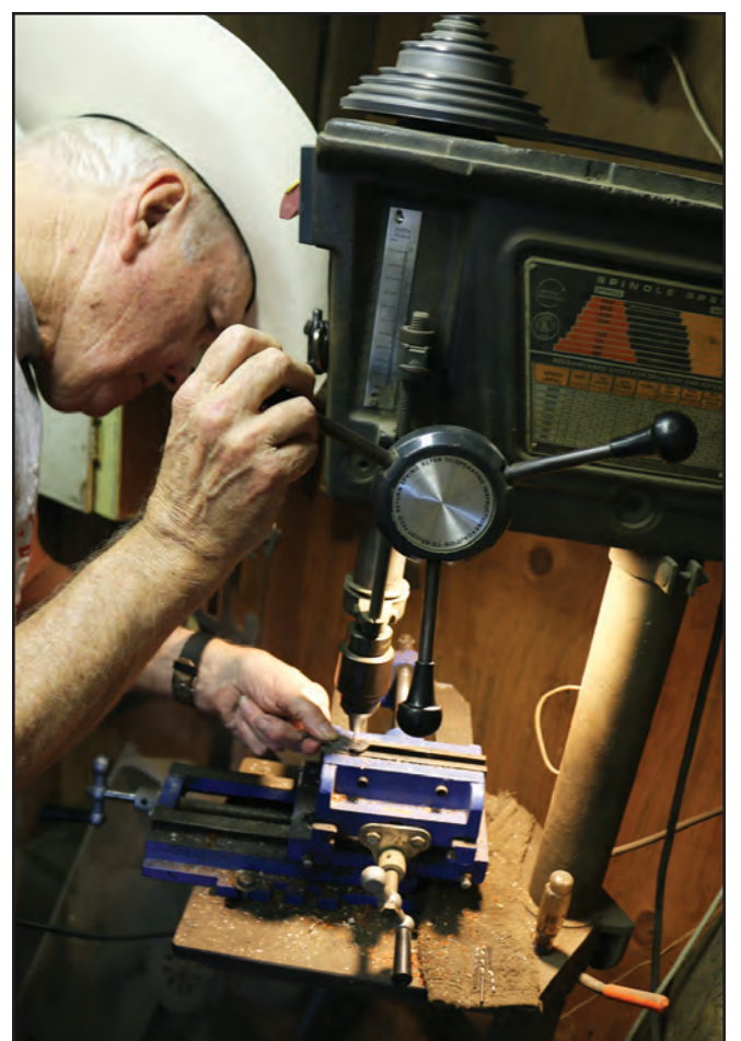
Bill Smith puts a divot on a blade so that it will snap into place. (PHOTO BY TIM FLEISCHER)
